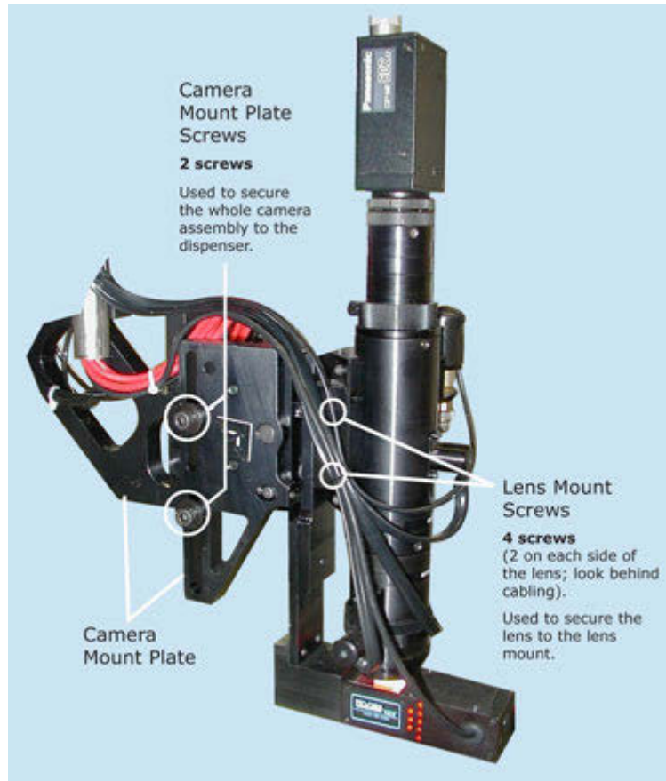
Figure 31: Screw locations for mounting Camera/Lens
