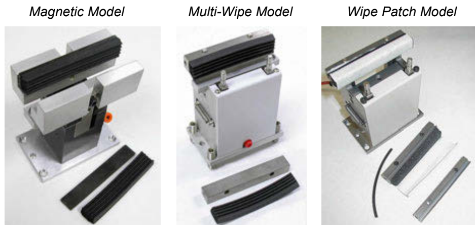
Figure 28: One jaw shown removed and disassembled from each model.
