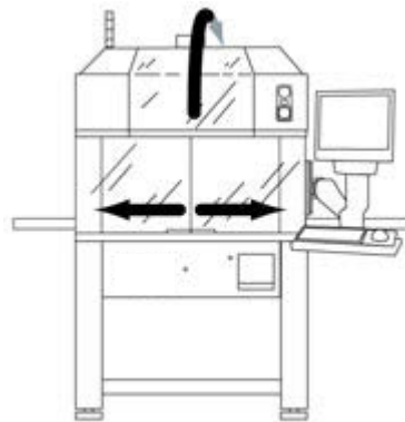
Safety shield opens upward & safety doors open to the sides
