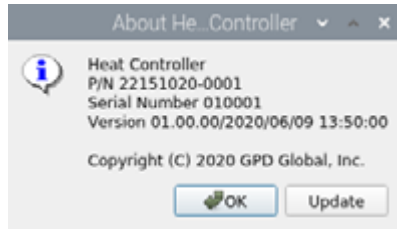
Figure 11: An UPDATE button is present when an update to the control software is available.
