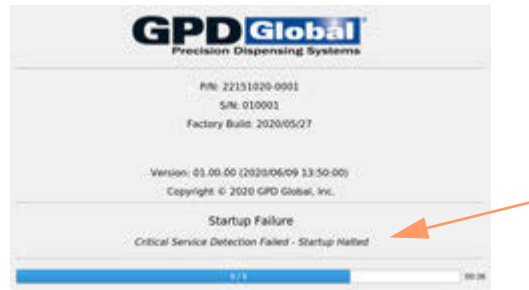
Figure 5: Example of failed start up.
