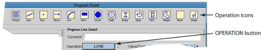
All *shapes* are also always available unless filtered by class. A list of all currently available (non-class filtered) shapes can be accessed with the ShList icon located at the left of the icon group (shown above), from the Select List window (shown below), or with the Program Detail OPERATION button.
